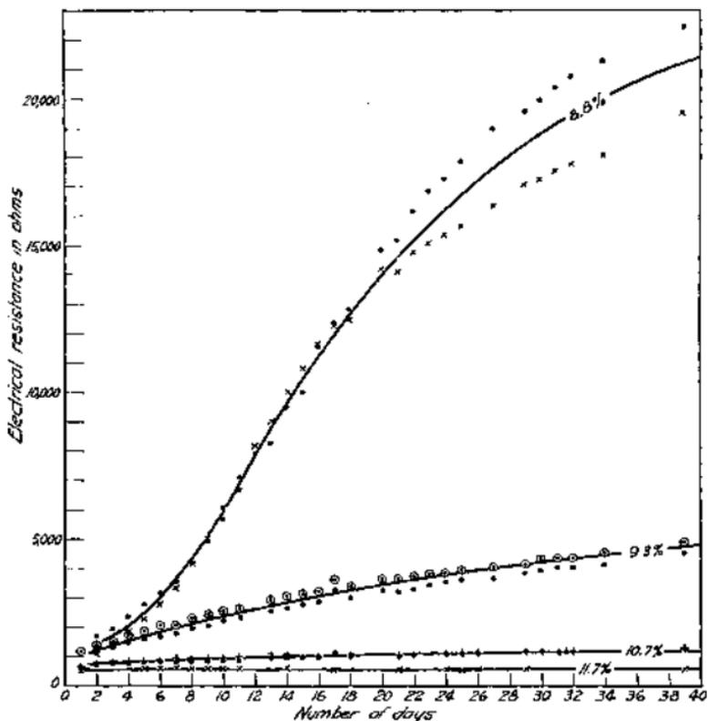
Figure 1.—Electrical resistance as a function of time when blocks are first saturated, and after having the excess water wiped off, are placed in Yolo fine sandy loam of the moisture content shown. The time required for equilibrium is obviously greater for the drier soils, and is appreciable even for higher contents.
