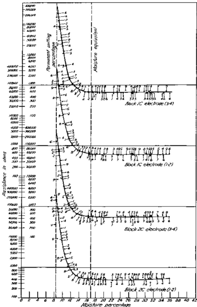
Figure 2.—Derived curves showing resistance of blocks as a function of moisture content when the blocks are placed in Yolo fine sandy loam upon which plants were growing in the laboratory. The numbers distributed along the curve indicate the cycle from which the data were obtained.
