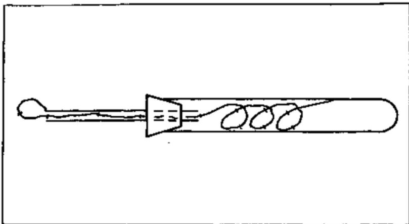
Figure 1.—Apparatus used for circumference measurements of beets.
