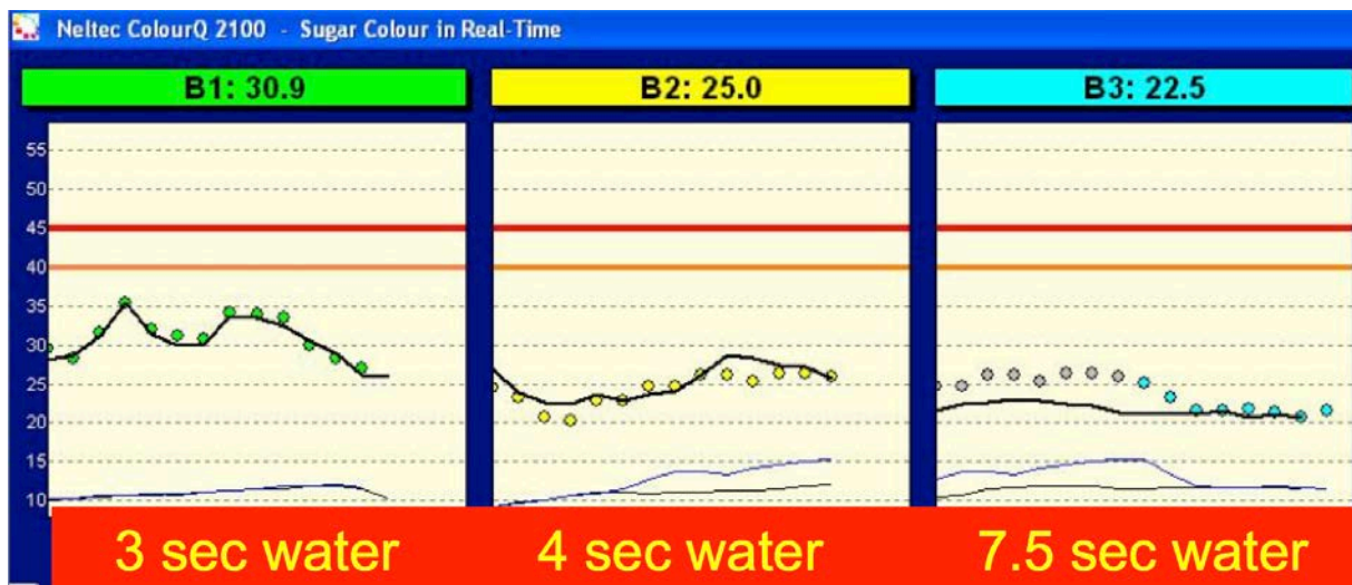
Figure 4 : Colour of sugar delivered by the centrifugals after reducing the spray time in Centrifugal B1 by 1 sec (and thus the volume of water used by 3 l).'
