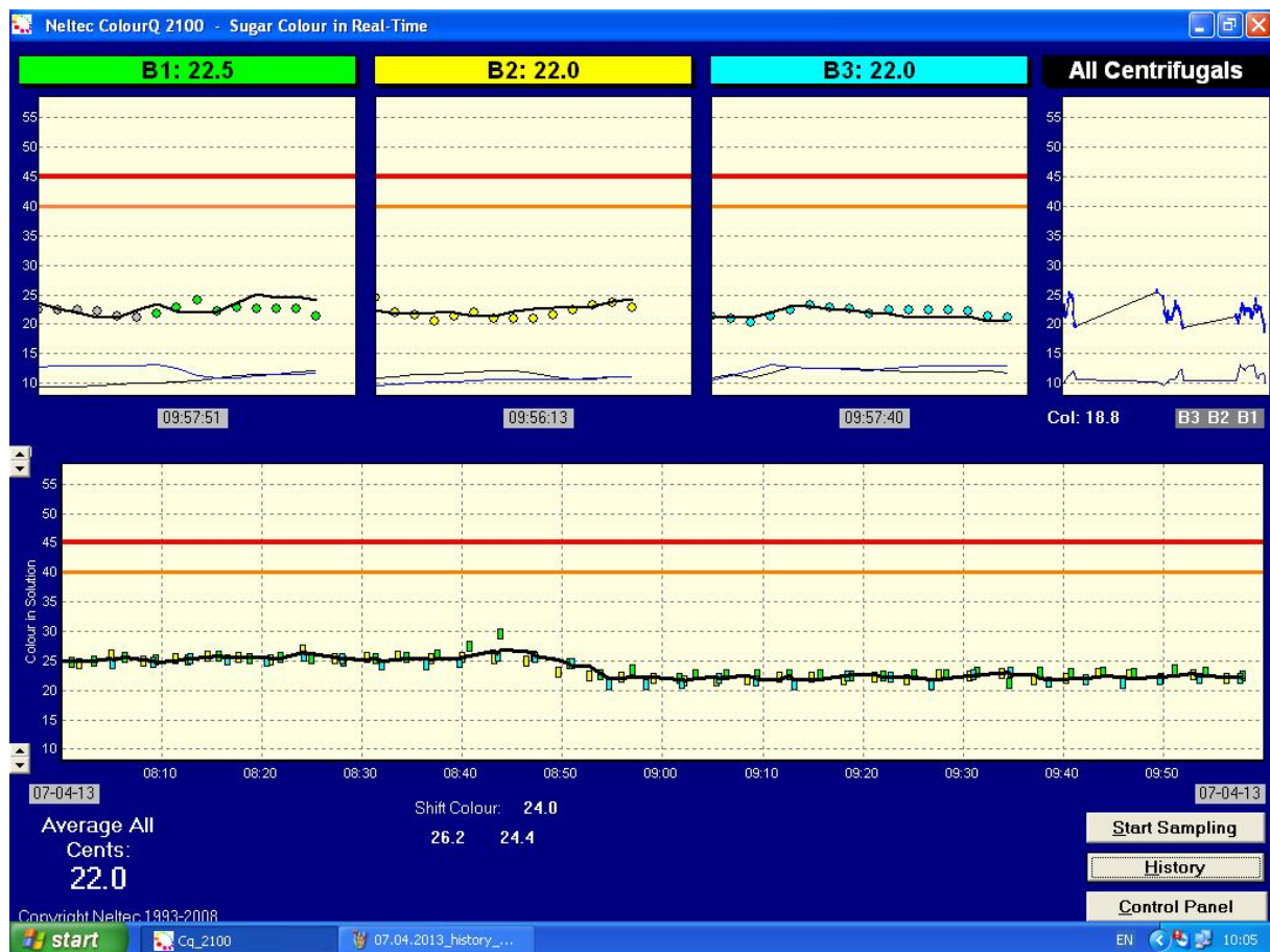
Figure 6: Display of average colour of sugar discharged by each centrifugal in each strike (lower chart).
