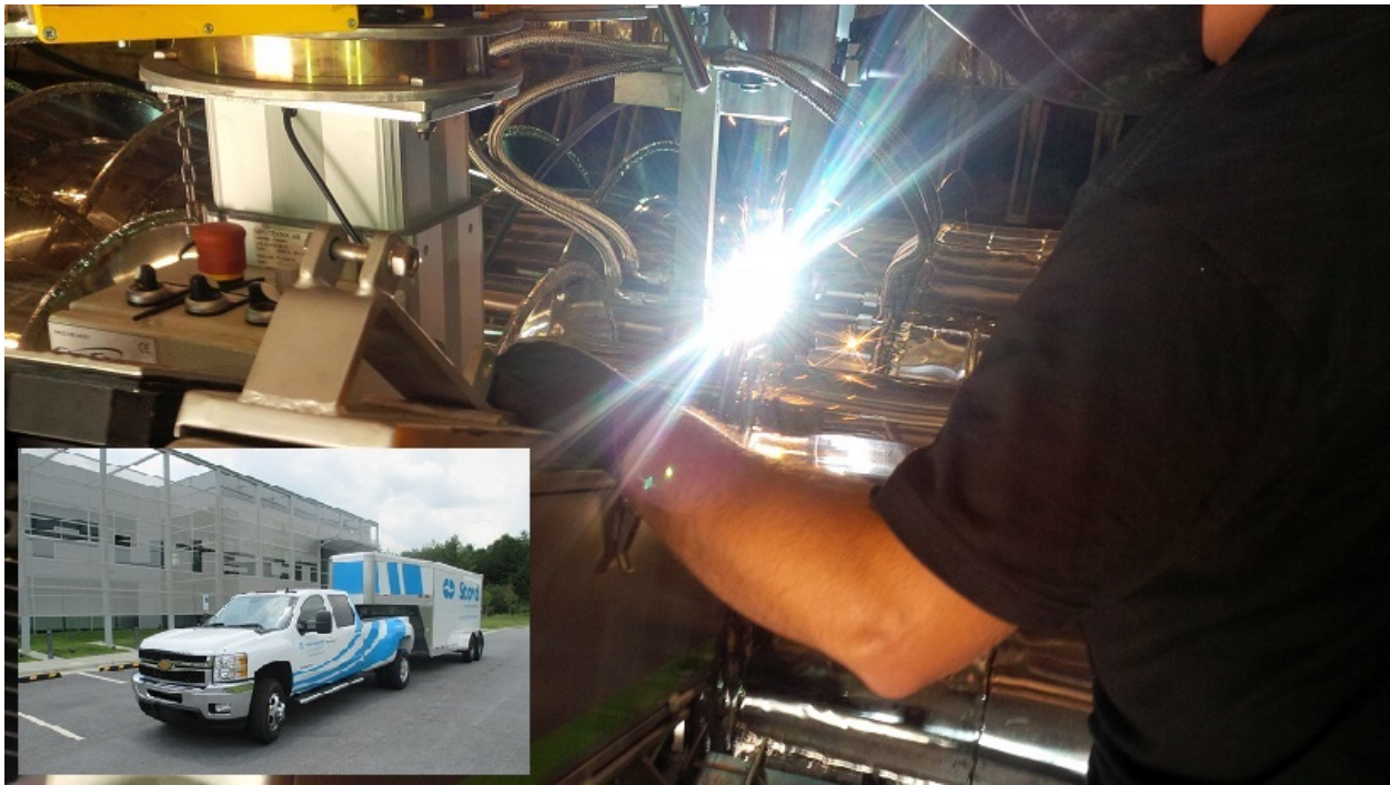
Figure 1: MIG welding fixture used by the Flightbuilder crew
