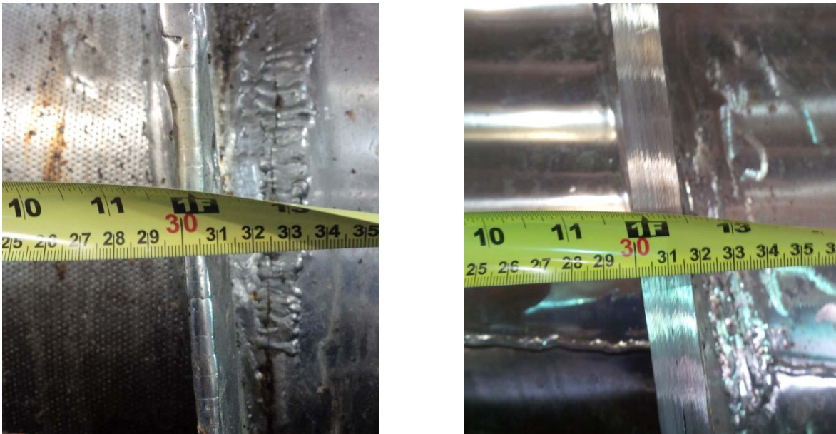
Figure 3: Left shows flighting tip of Stord 2500 press prior to rebuild. Right shows flighting tip post-rebuild.
